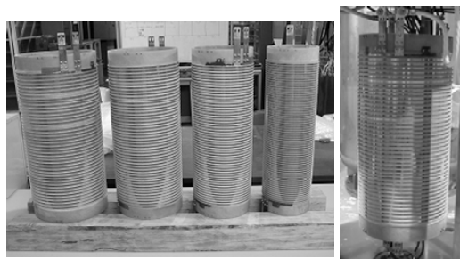
Fig. 3. Photo of the current limiting coil; each four layer(left) and assembled figure (right)
